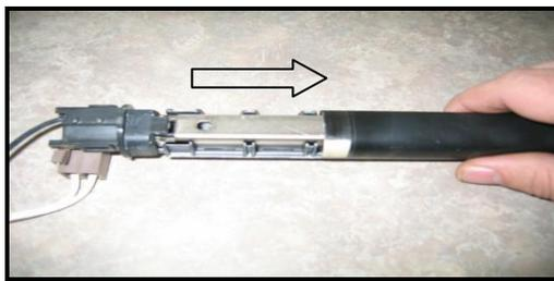
5. Remove the worn fixing film by sliding it off the rear of the heating element
